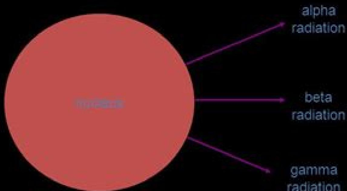
The behaviour of radioactive materials (radioactive decay) cannot be changed by chemical or physical processes
