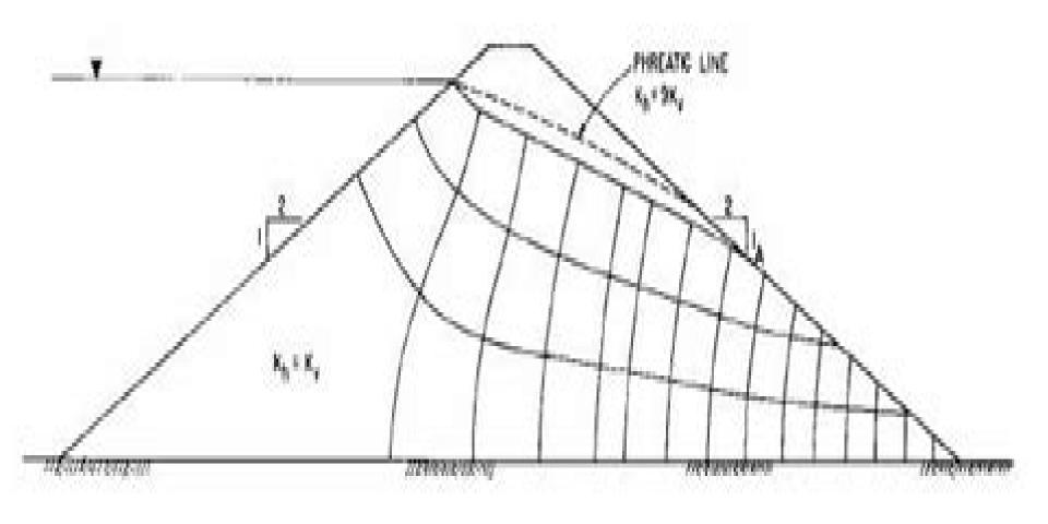
FLOW NET FOR HOMOGENEOUS DAM - NO UNDERDRAINS
