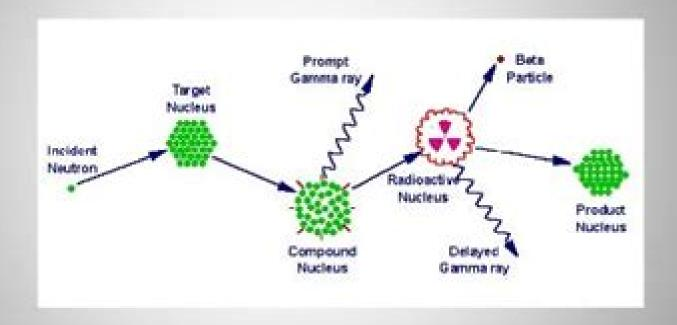
Fig. 1. Diagram illustrating the process of neutron capture by a target nucleus followed by the emission of gamma rays. The above figure is from http://www.missouri.edu/~glascock/nna\_over http://ww
