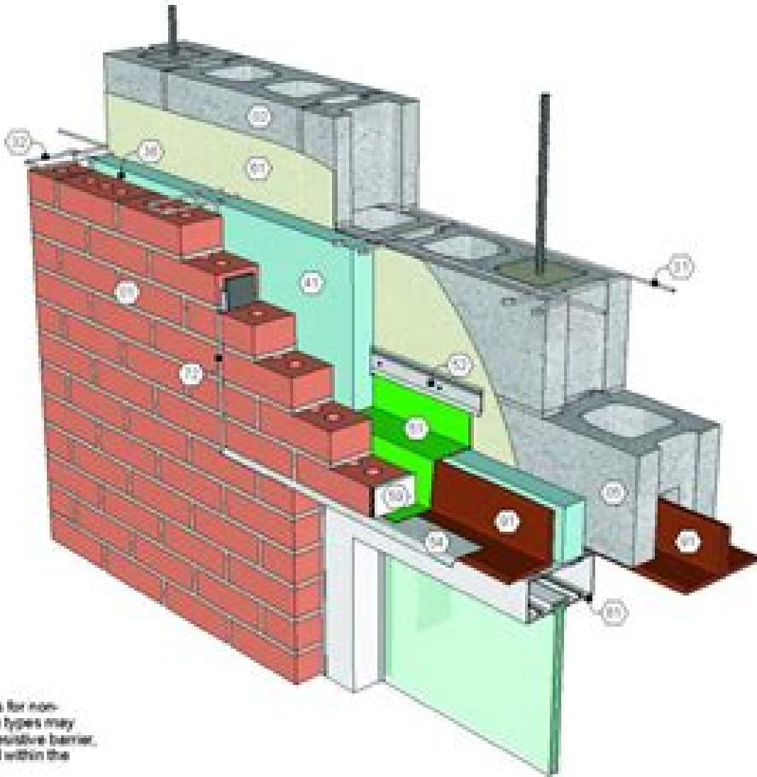
Note: Code requirements for non-combustible construction types may affect insulation, water-resistive barrier, and other materials used within the window head assembly.
