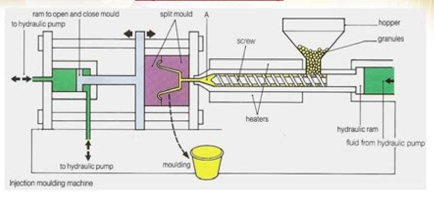
The screw is moved backwards, as it rotates, until a measured quantity of plastic is at position 'A'. The screw is then driven forwards by a hydraulic ram, injecting the molten plastic into the mould.
