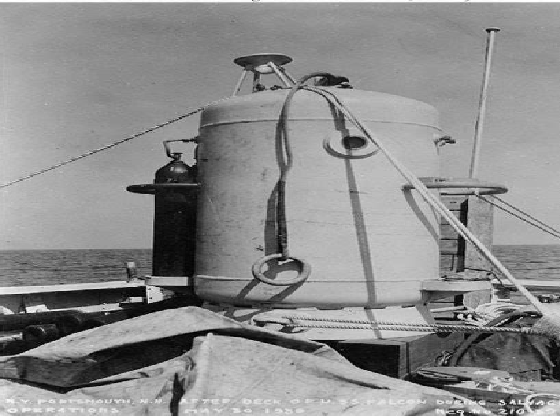
Photo # NH 57503 Diving bell on USS Falcon, 30 May 1939
