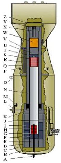
Cross-section drawing of Y-1852 Little Boy showing major mechanical component placement. Drawing is shown to scale. Numbers in () indicate quantity of identical components. Not shown are the APS-13 radar units, clock box with pullout wires, baro switches and tubing, batteries, and electrical wiring. (John Coster-Mullen)
