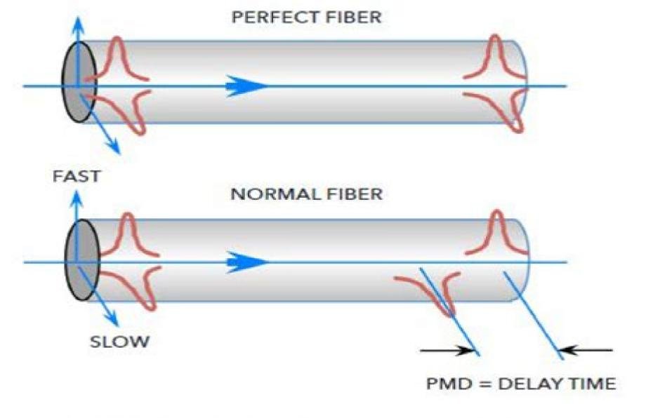
Polarization mode dispersion - delay in the two polarizations traveling down a fiber.
