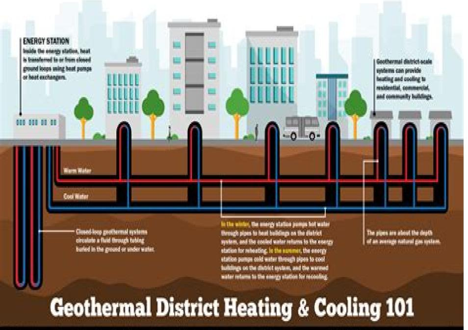
This illustration is one configuration of a geothermal district heating and cooling (CDHC) system, in this case using geothermal heat pumps. There are many other GDHC solutions that might also work for your community.
