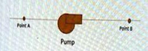
60 deg F water is being pumped to the right through piping. Gage pressure at point A is 20 psi while gage pressure at point B is 20 psi as well. Points A and B are at the same elevation. It's steady-state and the piping is all the same diameter so the water speeds and A and B are the same. Piping friction losses from A to B are 76.7 ft\*lb/slug.
