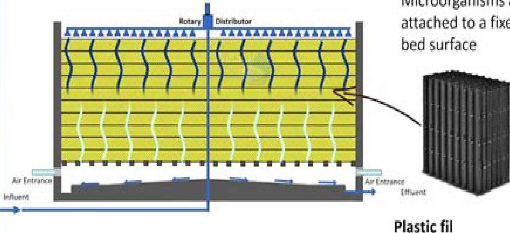
Understanding the Process of Trickling Filters Via Diagram
