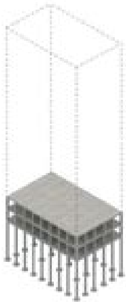
Concrete structure on steel column foundation
