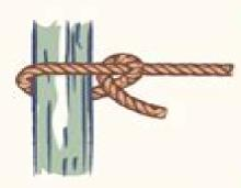
This quick and easy knot is the basis for many other nautical knots. While it isn't reliable on its own, it can be used to secure the end of a line when tying other knots.
