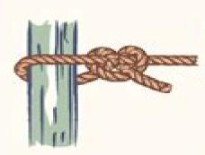
This is a more secure version of the half hitch and is used to tie to pilings or mooring rings. It's a good option for keeping boats secure in their slips long-term.
