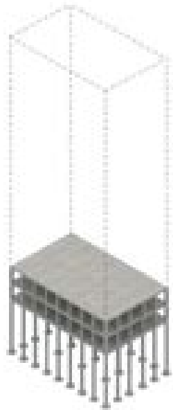
Concrete structure on steel column foundations
