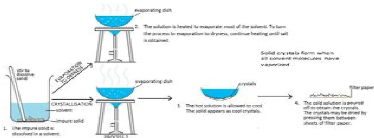
Crystallization is a process used to separate a solid in liquid mixture where the solid is soluble in the solvent and dissolves in it and forms a homogeneous solution. Example: A mixture of NaCl and water.
