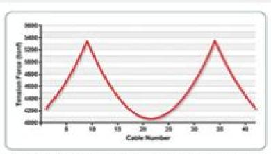
Initial tension forces in cables of a suspension bridge
