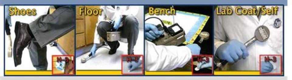
Use the contamination swipe method when handling H-3.
