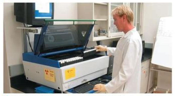
3 The test tubes are placed in a scintillation counter.
