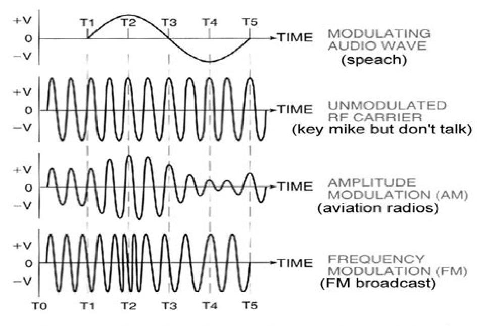
Modulation: from T0 to T1, carrier frequency is unmodulated; from T1 through T5, audio wave modulates carrier frequency.
