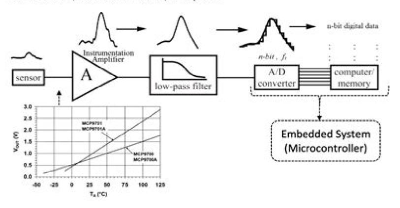
This system is used to monitor temperature of a 1000-liter water tank for an industrial process control. Our microcontroller has a 5V power supply and two 10-bit ADCs with maximum sampling rate of 50 kHz.
