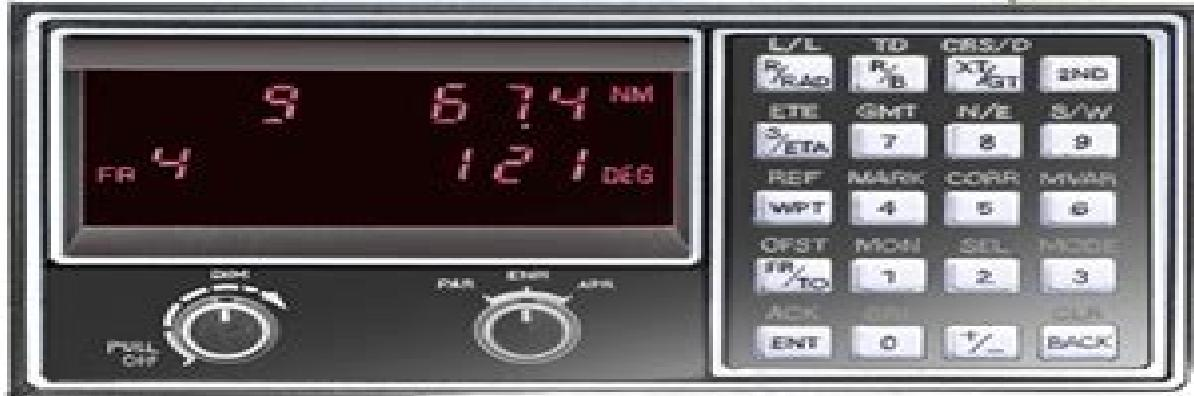
A microprocessor allows navigation to specific fixes or routes
