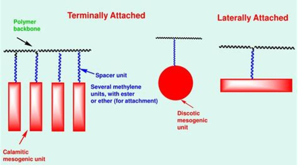
A general template for side chain liquid crystal polymers
