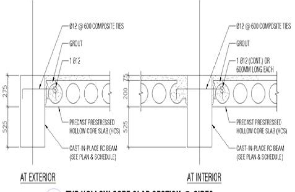
TYP.HOLLOW CORE SLAB SECTION @ SIDES 0.8003
