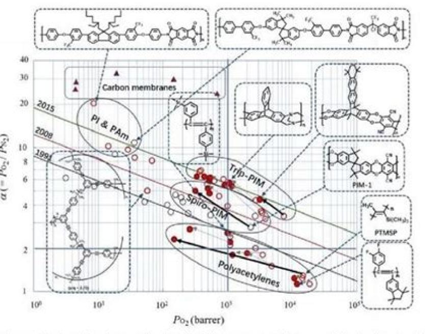
Upper plots through polymers showing the highest  $\alpha$  at each  $Po_2$  reported in the literature in 2020 ( $\bullet$  after aging,  $\odot$ : before aging).
