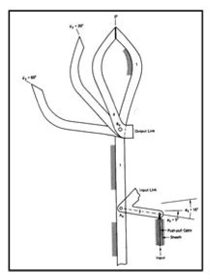
A four-bar function generation mechanism to lower an attic stairway.
