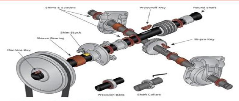
Mechanical Power Transmission is the transfer of energy from its source to another location using mechanical elements.
