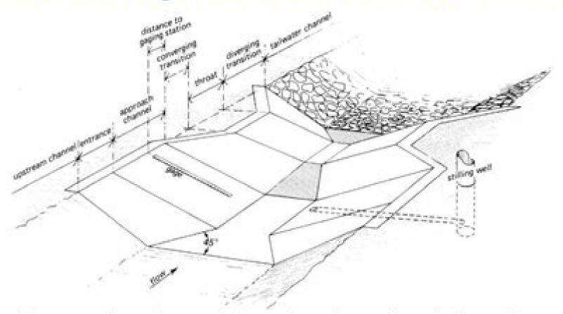
The term *long-throated flume* describes a broad class of critical-flow flumes and broad-crested weir devices used to measure flow in open channels.
