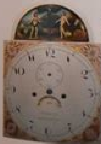
(xi) Andrew of Newnham, Gloucestershire, is an unknown clock maker. This is a Walker and Hughes of Birmingham automatic dial c. 1812 where the background of the Garden of Eden is a separate engraved piece and only five's are moved. The contents are definitely Walker work with their respective diamond shapes. An inclusion layer was stuck on at the centre of each oval. There is one other known dial for the same dial maker using an inclusion layer, but neither dial maker seems to have used this decoration.
