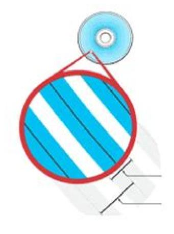
0.6µm Track Width 1.6µm Track Distance (Pitch)
