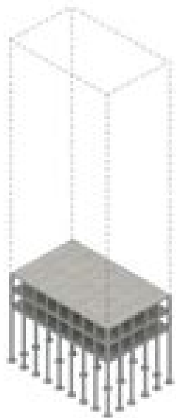
Concrete structure on steel column foundations
