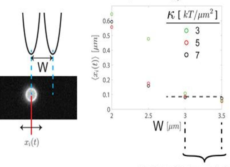
Range of trap separation, W<sub>trap</sub>, with minimal trap-trap interactions
